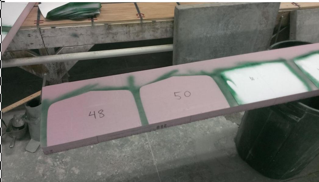
Paper templates transferred onto foam.
