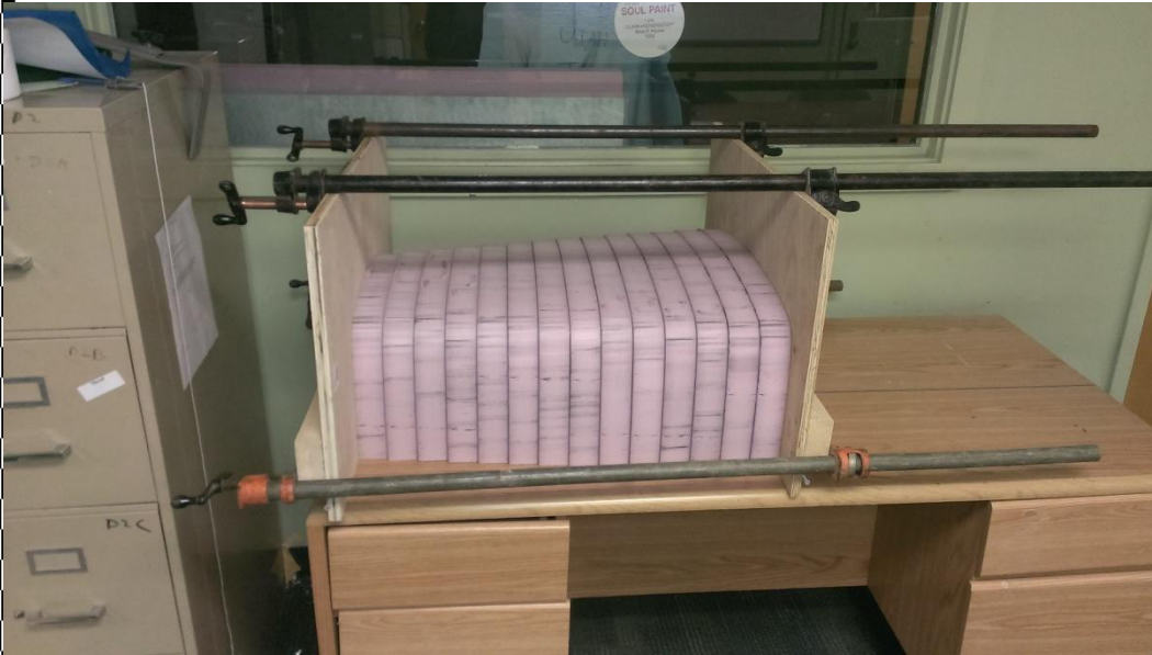
Clamping glued 2 foot foam section together.
