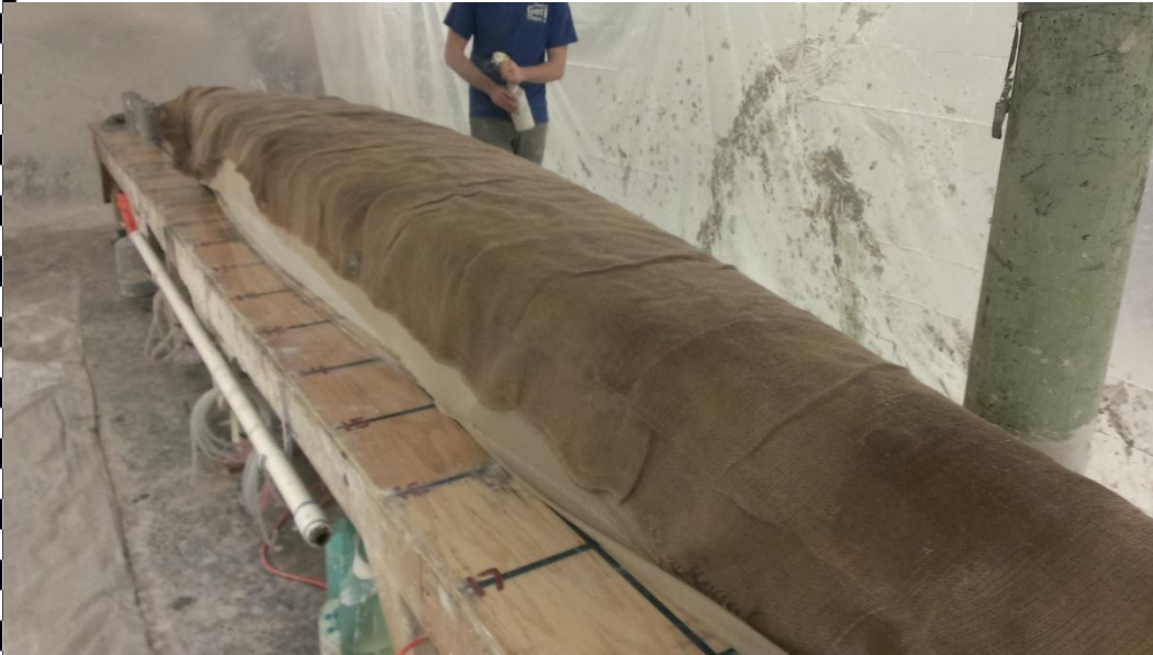
Canoe covered in burlap to help assure a moist cure.
