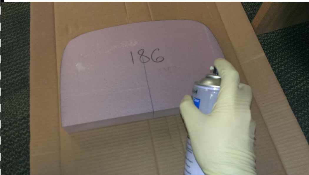
Applying glue to foam section.
