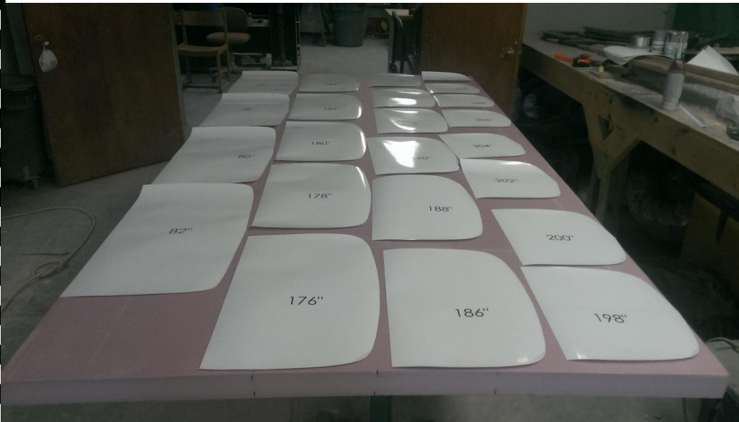
Laying out paper templates to be cut into foam sections.
