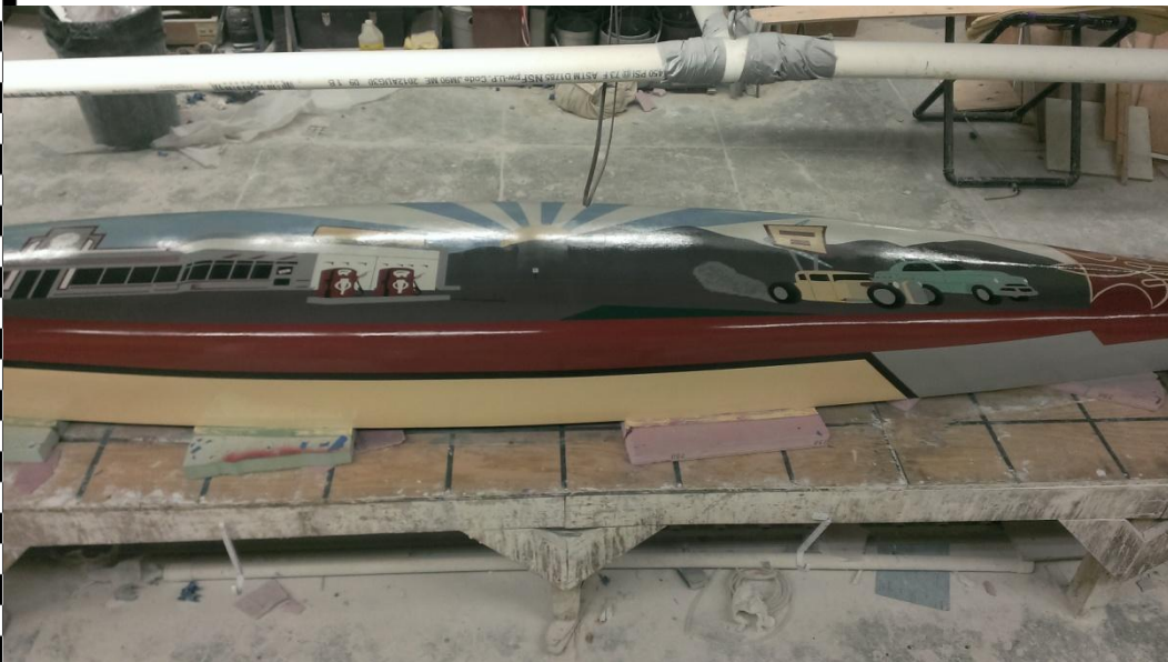
Hull after first coat of sealer.
