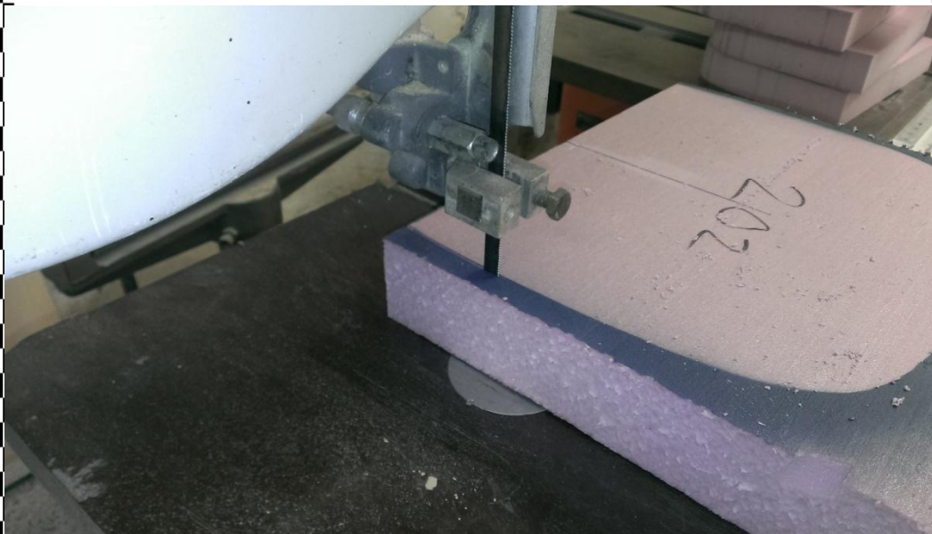
Foam sections are cut on a band saw.
