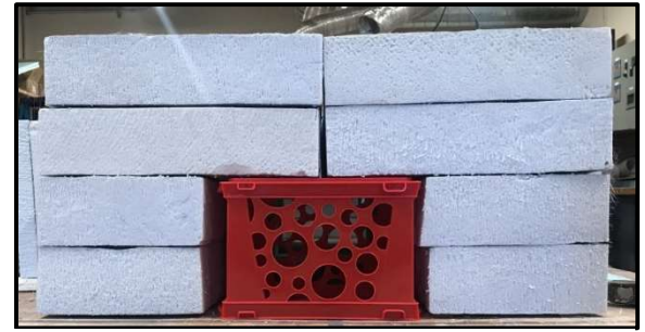
Figure 1: Construction of Recycled Foam Composite Mold (Pre-Milling)
