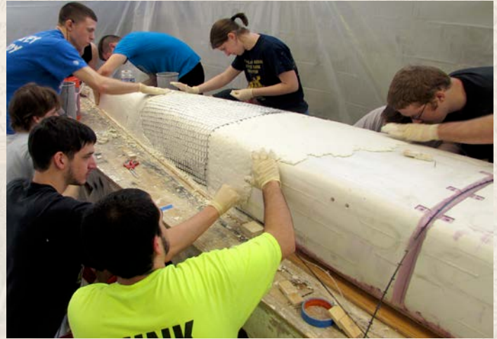
Figure 8. Concrete and Reinforcement Placement
