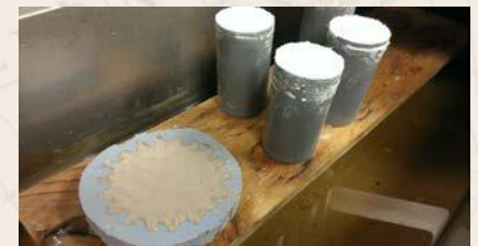
Figure 5. Steam Cured Elements
