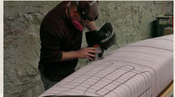
Figure 6. Routing of Channels
