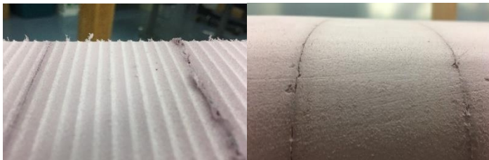
Figure 7. Comparison of Machine Finish vs. Sanded Finish
