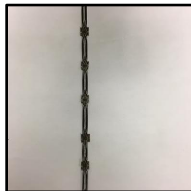
Sample 3: Strand of Basalt used for Ribs and Gunwales
